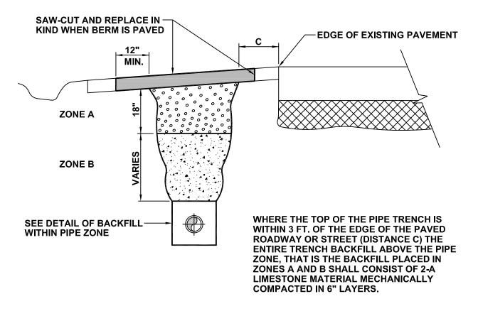
WHERE THE TOP OF THE PIPE TRENCH IS GREATER THAN 3 FT. FROM THE EDGE OF THE PAVED ROADWAY (DISTANCE C) BACKFILL PLACED IN ZONE B SHALL BE EXCAVATED MATERIAL FROM THE TRENCH, FREE OF ROCKS LARGER THAN 3" AND MECHANICALLY COMPACTED IN 6" LAYERS. BACKFILL MATERIAL PLACED IN ZONE A (THE TOP 18" OF THE TRENCH) SHALL BE 2-A LIMESTONE MATERIAL MECHANICALLY COMPACTED IN 6" LAYERS.
