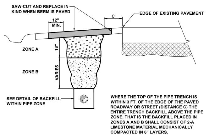
WHERE THE TOP OF THE PIPE TRENCH IS GREATER THAN 3 FT. FROM THE EDGE OF THE PAVED ROADWAY (DISTANCE C) BACKFILL PLACED IN ZONE B SHALL BE EXCAVATED MATERIAL FROM THE TRENCH, FREE OF ROCKS LARGER THAN 3" AND MECHANICALLY COMPACTED IN 6" LAYERS. BACKFILL MATERIAL PLACED IN ZONE A (THE TOP 18" OF THE TRENCH) SHALL BE 2-A LIMESTONE MATERIAL MECHANICALLY COMPACTED IN 6" LAYERS.
